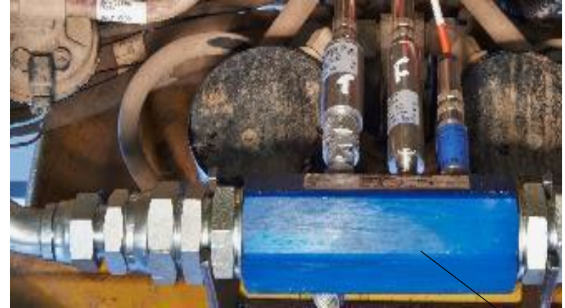
Hydraulic flow meter
